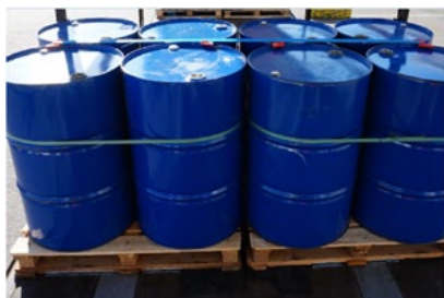
Zwei Drumclips pro Ladeeinheit / Two Drumclips per load unit
