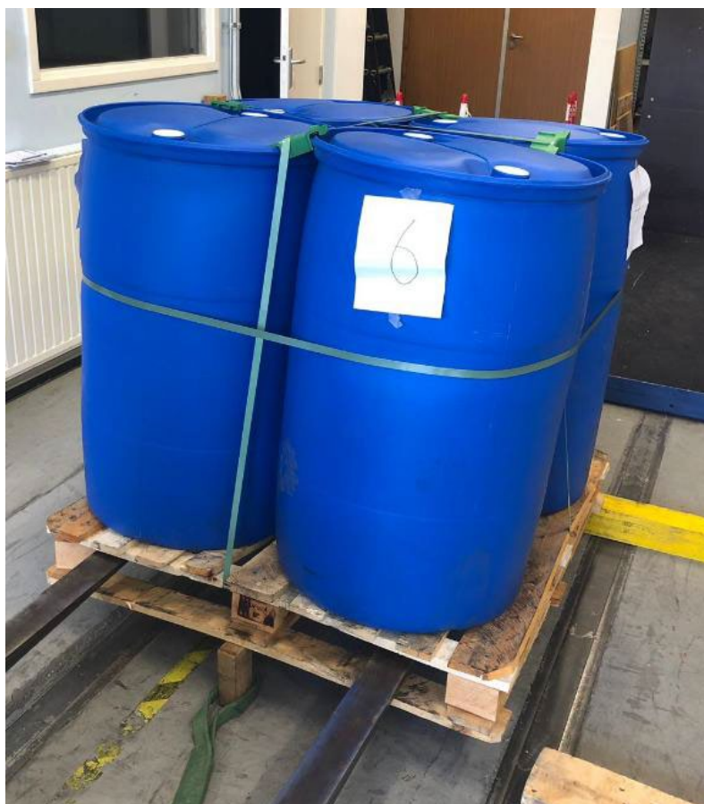
Figure 8. Position of drum clips during drop testing.
