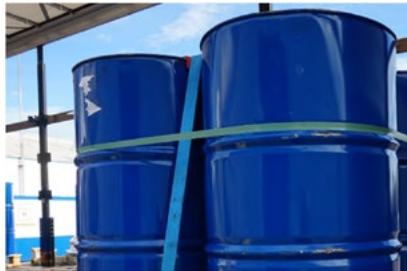
Variante 5a: Spanngurt hinter dem Strap / Variant 5a: Lashing belt behind the strap
