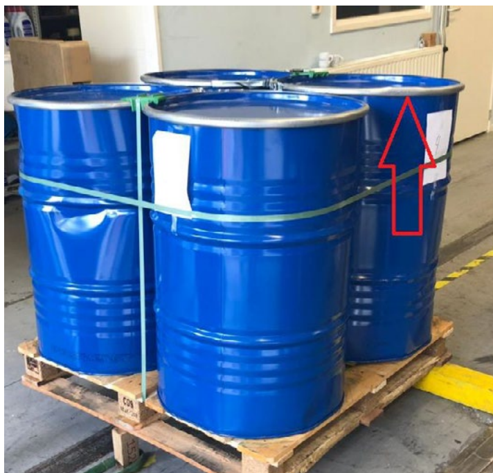
Figure 8. Damage to drum ring; only face 4.
