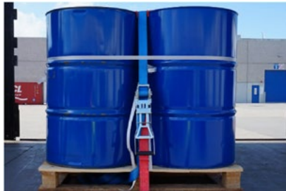
Horizontaler und vertikaler Cordstrap®, Spanngurt hinter dem horizontalen Cordstrap® / Horizontal and vertical Cordstrap®, lashing belt behind the horizontal Cordstrap®
